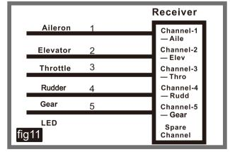
Attach the aileron servo leads to the previously installed "Y" harness. Elevator servo lead goes to elevator channel of your receiver. The rudder servo goes to the rudder channel. Attach the ESC connector to the throttle channel of the receiver.
